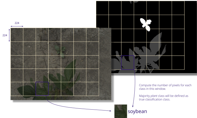
Figure 1. Demonstration of how the original WE3DS segmentation images are divided into smaller classification images.
