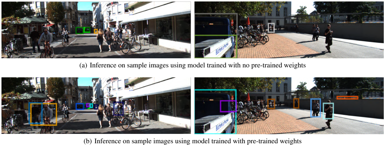
Figure 13: Visualizing the impact of pre-trained weights on previously unseen and novel objects that are not part of the training dataset.
