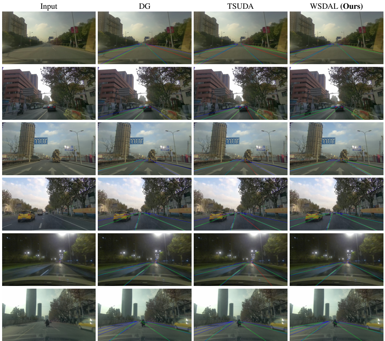
Figure 9. Qualitative results on the task CULane \rightarrow CurveLanes from CLRNet with ResNet-18 backbone. We demonstrate the ability to eliminate the false positive predictions driven by WSDAL. We show the true positive predictions in green, false positive predictions in red, and ground truth in blue.
