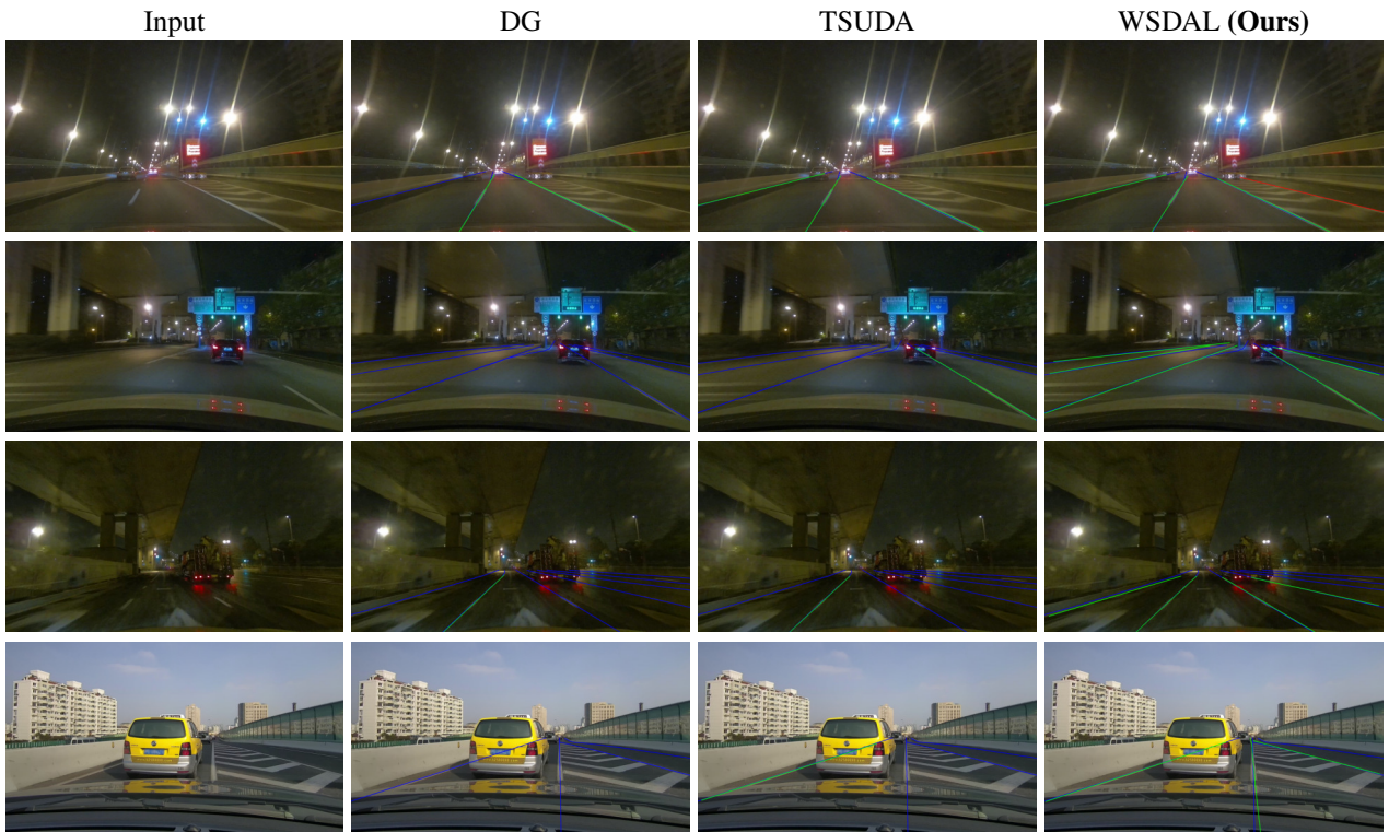
Figure 11. Qualitative results on the task CULane \rightarrow CurveLanes . We observe that there are also inconsistent annotation policies that may affect the NoL-based adaptation process. We show the true positive predictions in green, false positive predictions in red, and ground truth in blue.
