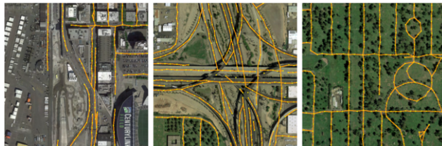
Figure 7. Some error patterns. Left: geometry decoder missed the road segment in the middle. Middle: topology decoder missed connections in a complex interchange. Right: an interesting case where SAM-road predicts the trails in a park which are not part of the label.
