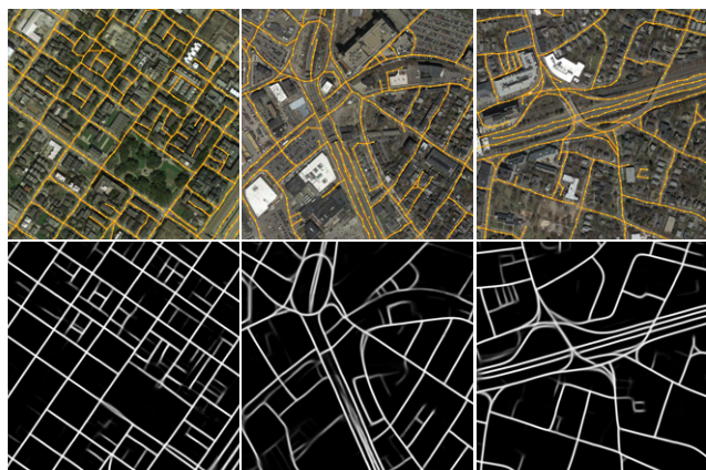
Figure 1. SAM-Road effectively predicts accurate road network graphs for dense urban regions, including roads with complex and irregular shapes, bridges, and multi-lane freeways. The corresponding segmentation masks are sharp and clear.
