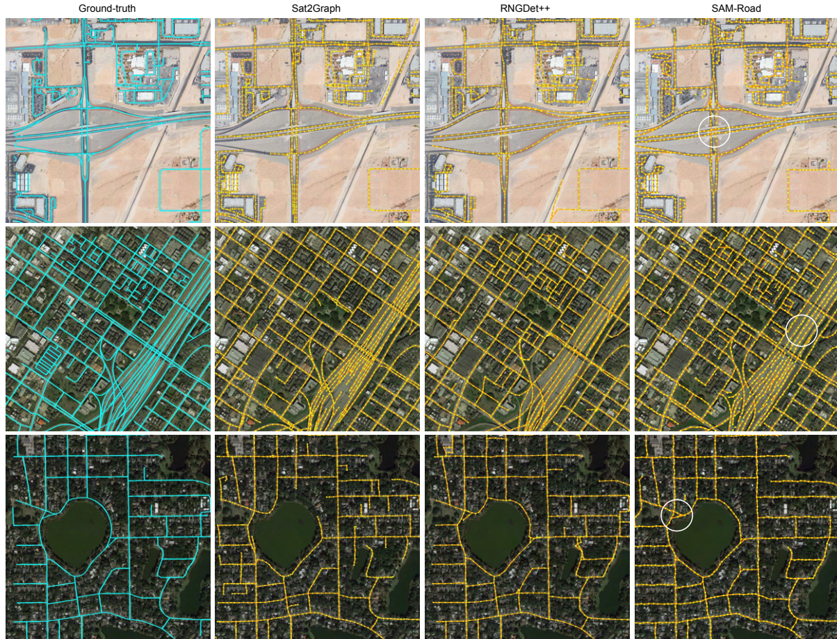
Figure 5. The visualized road network graph predictions of SAM-Road and two baseline methods. Better zoom-in and view in color. Overall, SAM-Road generates highly accurate predictions. The circles highlight especially challenging spots: in the first area, SAM-Road correctly predicts the overpass structure. In the second one, SAM-Road gives superior results for the parallel freeways. The third spot shows an irregular intersection where the two baselines fail.
