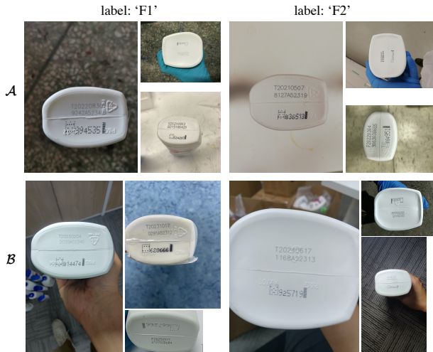
Figure 2. Sample images of the bottom side of commercial products produced by two manufacturers, ‘F1’ and ‘F2’, in pre-existing ( \mathcal{A} ) and newly released ( \mathcal{B} ) datasets. Target regions (dotted parts) to be segmented by U-Net [48] in Sec. 2.2) with ever-evolving anti-counterfeit code patterns embody spatial variations led by varying illumination, camera bias [20], and noisy textures [21] (e.g. dust and stains), affecting the overall FGVC accuracy.
