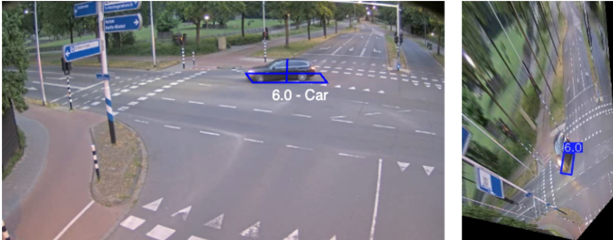
Figure 2. The agents are initially detected in the camera view. YoloV8 estimates a bounding box for each agent, assigns to it an ID, and tracks it across frames. Subsequently, the detected bounding boxes are projected in the BEV, where the three dimensional bounding boxes are detected, carrying over the id assigned to the agent in the camera view.
