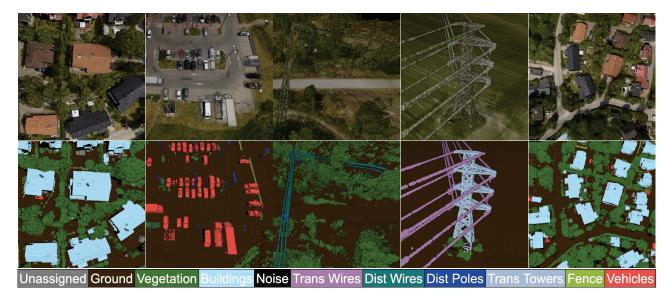
Figure 1. **Overview of the proposed ECLAIR dataset.** We introduce ECLAIR, a new outdoor large-scale aerial LiDAR dataset. It covers a total area of more than 10 square kilometers encompassing 11 semantic classes. The long-tail accurate annotations enable fine-grained semantic understanding. Different semantic classes are labeled by different colors.
