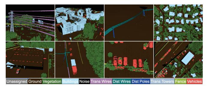
Figure 7. **Qualitative results of the best model.** We assess segmentation performance of the strongest baseline model on the test split of the proposed ECLAIR dataset. The top row demonstrates successful cases where the model performs well. In contrast, the bottom row highlights failure scenarios where the model produces noisy, inaccurate predictions.
