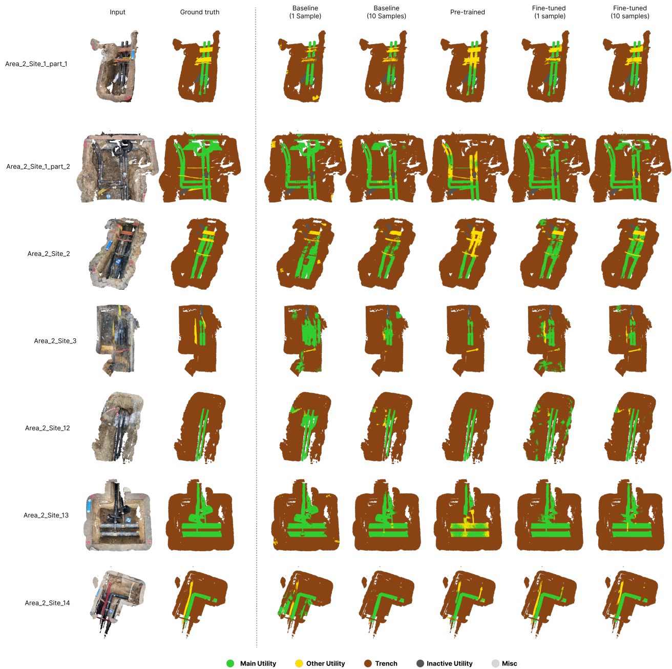
Figure 3. Qualitative Examples from running inference on samples from Heating Area 2 with 5 trained PointNeXt model versions: 2 models which are trained on 1 and 10 samples from Heating Area 1 (called Baseline), 1 model pre-trained on samples from Water Area 1-4 and 1 model pre-trained on samples from Water Area 1-4 and fine-tuned with 1 and 10 samples from Heating Area 1.
