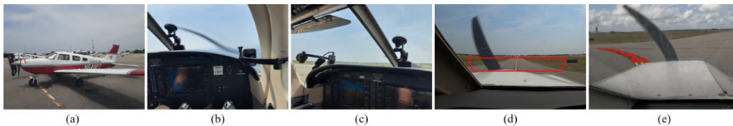
Figure 1. (a) Illustrates the aircraft used for this research, (b) and (c) displays the setup of cameras at different perspectives inside the aircraft, (d) shows the manually defined region of interest on a frame, (e) showcases the annotation label created by ALINA on a frame.
