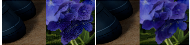
(b) Raytrace Samples variations on shadow quality in rendered images. Left: 1. Right: 32
