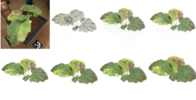
Figure 9. Coltsfoot point cloud reconstruction. Notice the changes in stem thickness. Top left: cleaned point cloud with point size 0.2. From left to right, top to bottom are reconstructions of point sizes: 0.01, 0.1 0.2, 0.6, 1.0, 2.0, and 5.0.
