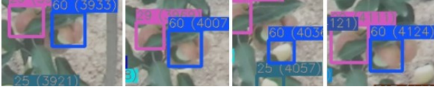
Figure 5. Closeup over two adjacent detections on frames 60-63 from Galafab-west dataset. The blue detection is tracking a fruit on a tree, but is switched to a fruit on the ground in the third frame.
