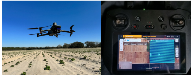
Figure 2. Mavic 3 Multispectral drone in flight on the left, and flight parameters on the right
