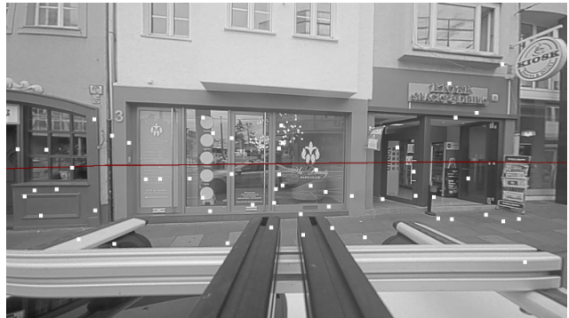
Figure 1. Typical point reflections (white squares) from radar overlaying image from camera: Limited object definition in radar creates poor conditions for driving set matching in DETRs
