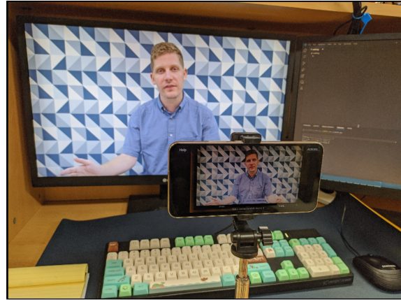
Figure 2. Moiré Pattern-impacted Dataset Generation: The setup is to display videos from various datasets on a computer screen. These videos are captured using a smartphone camera, leading to the recording of the authentic Moiré pattern that appears on the computer screen.
