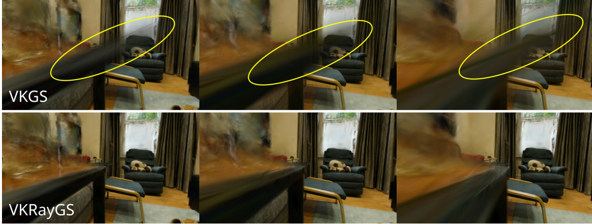
Figure 5. Artifacts one might experience with GS models (top) as opposed to RayGS (bottom), while moving close to objects. Renderings are from the room scene of MipNeRF360 and obtained with VKGS and our VKRayGS, respectively.
