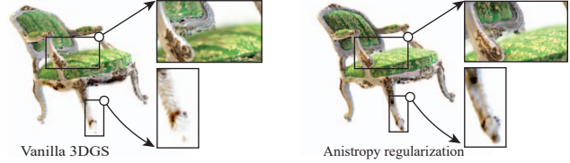
Figure 4. Anisotropy regularization. Anisotropy regularization effectively maintains rendering quality under large deformations. Without the regularization term, 3DGS tends to generate fuzzy and spiky artifacts, especially near the surface of the model (left). When the regularization is applied, image quality is greatly improved with correct specular effects.
