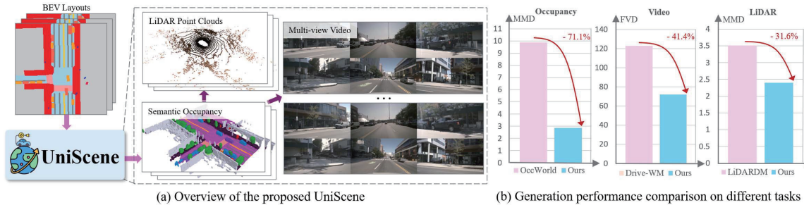
Figure 1. (a) Overview of UniScene. Given BEV layouts, UniScene facilitates versatile data generation, including semantic occupancy, multi-view video, and LiDAR point clouds, through an occupancy-centric hierarchical modeling approach. (b) Performance comparison on different generation tasks. UniScene delivers substantial improvements over SOTA methods in video, LiDAR, and occupancy generation.
