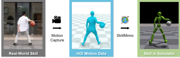
Figure 2. Concept of SkillMimic. We define an interaction skill as a set of Human-Object Interaction (HOI) state transitions that align with the intended skill semantics. These state transitions can be derived from captured HOI motion clips. If a simulated humanoid can manipulate objects such that the resulting HOI state transitions closely match those of the reference, we consider the humanoid to have successfully learned the interaction skill.
