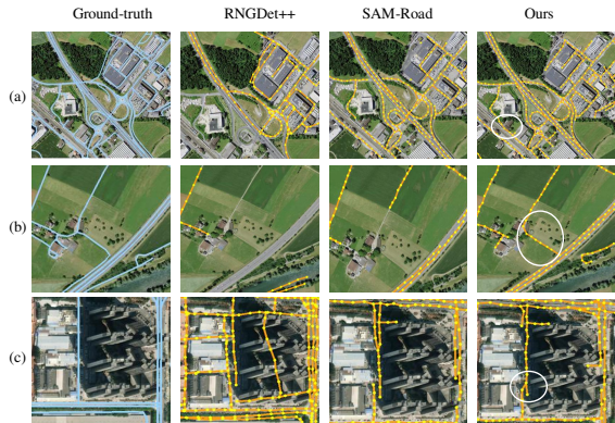
Figure 6. Visualisation of the different methods on the out-of-domain test set. In the rural road region with farmland as context ((a) and (b)), our method successfully avoids road disconnection. In the road region (c) with the shadow of a tall building, our proposed “extended-line” strategy accurately predicts the connectivity of the shaded portions.
