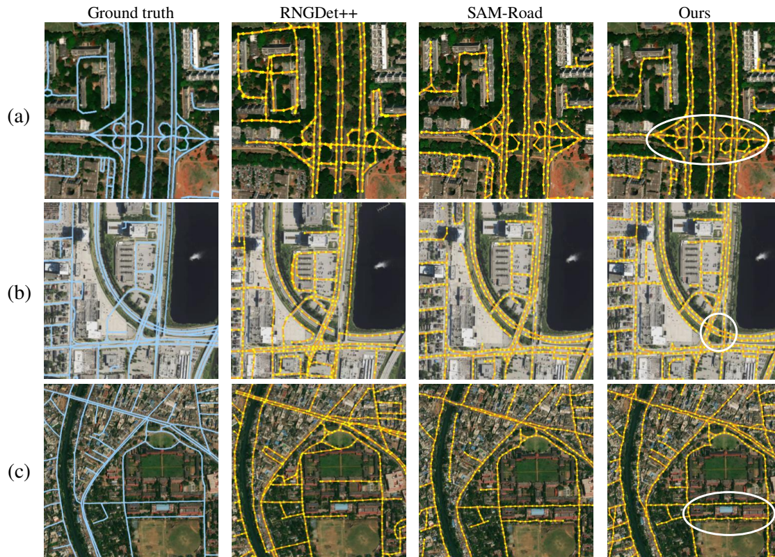
Figure 5. The visualized road network graph predictions of SAM-Road++ and two baseline methods. Better zoom-in and view in color. Overall, the prediction accuracy of SAM-Road++ is higher. In the crossroads regions (a and b), SAM-Road++ successfully predicted the complexity of multiple roundabouts and overpasses, and in predicting the tree-shaded region c, SAM-Road++’s prediction result is also more complete compared to the other two baselines.
