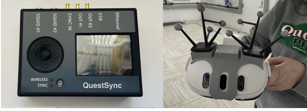
Figure A. Left: the QuestSync device. Right: Meta Quest 3 with two marker trees attached.
