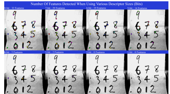
Figure 5. Features detected when using descriptors of various sizes
