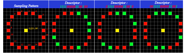
Figure 2. Examples of descriptors using a rotationally symmetric sampling pattern. The sampling pattern shown on the left is for 16-bit descriptors, and involves comparing 16 pairs of pixels, each comparison is between the central pixel and a pixel taken from a ring around this centre. Three descriptors are shown, each one is the right bit-shift of the previous. Note how this effectively rotates the visual structure the descriptor represents, as illustrated by the red (0s) and green (1s) on the pixel pairs of the sampling pattern.
