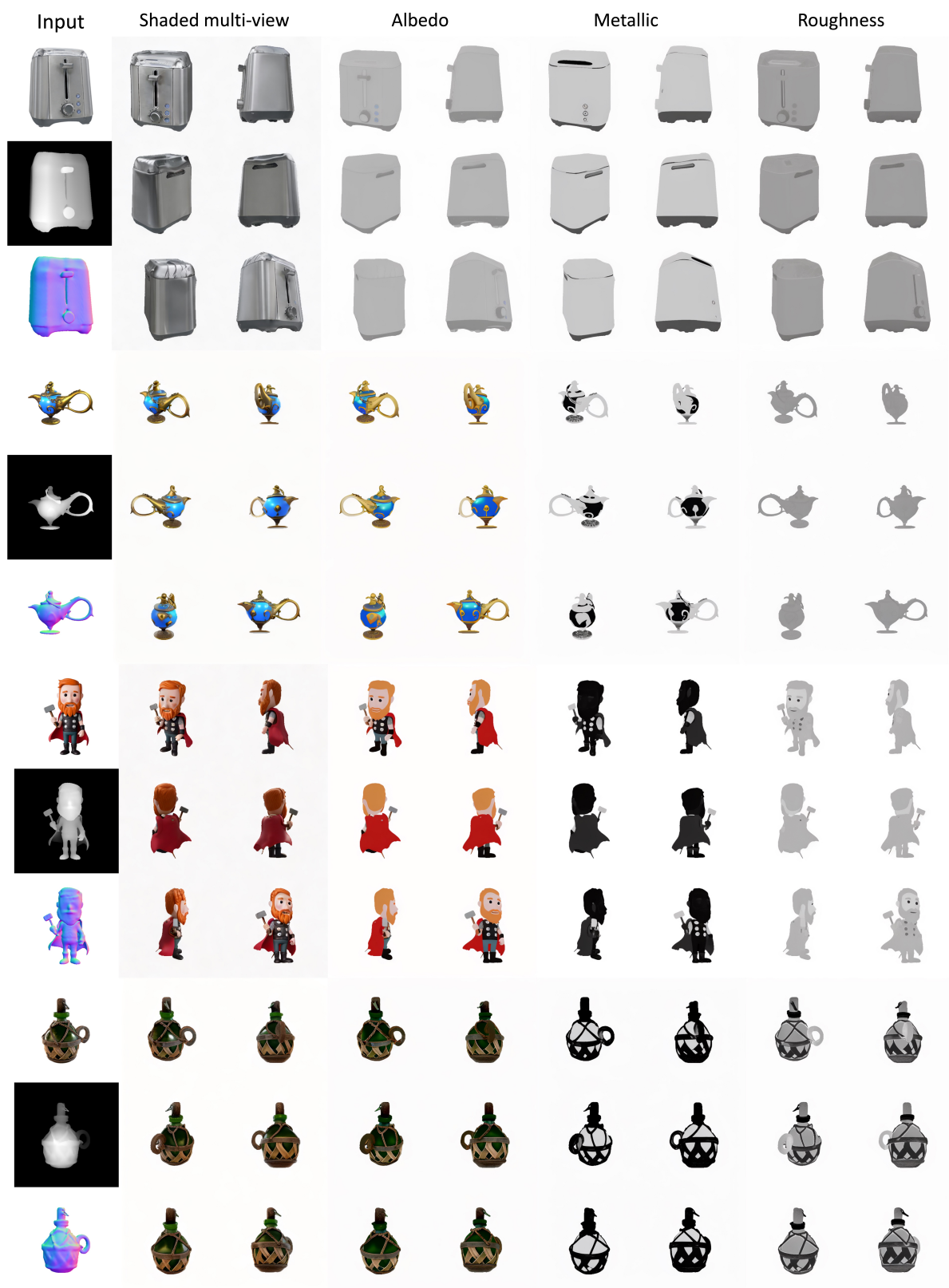
Figure 17. Intrinsic channels estimated using our multi-view PBR decomposer. The proposed PBR decomposer can handle images with complicated material under different lighting conditions.
