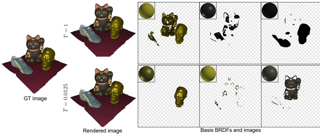
Figure 1. Impact of softmax function with low temperature. Low temperature softmax function results in interpretable basis BRDFs and images. We employ T = 0.0125 in our experiment.
