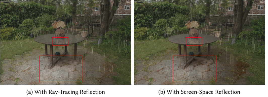
Fig. 11. Garden Scenario. Compared to ray-traced reflection rendering (a), SSR-based reflection rendering (b) achieves nearly identical visual quality while offering significantly higher efficiency and reduced memory consumption. The reflection regions are highlighted with red boxes.
