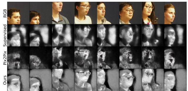
Figure 2. Thermalization results for side RGB images without paired thermal images from the TUFTS [17] database without regularization ( \lambda_W = 0 , \lambda_R = 0 ), Pix2Pix and our final model ( \lambda_W = 0.001C , \lambda_R = 1 ) (top to bottom).
