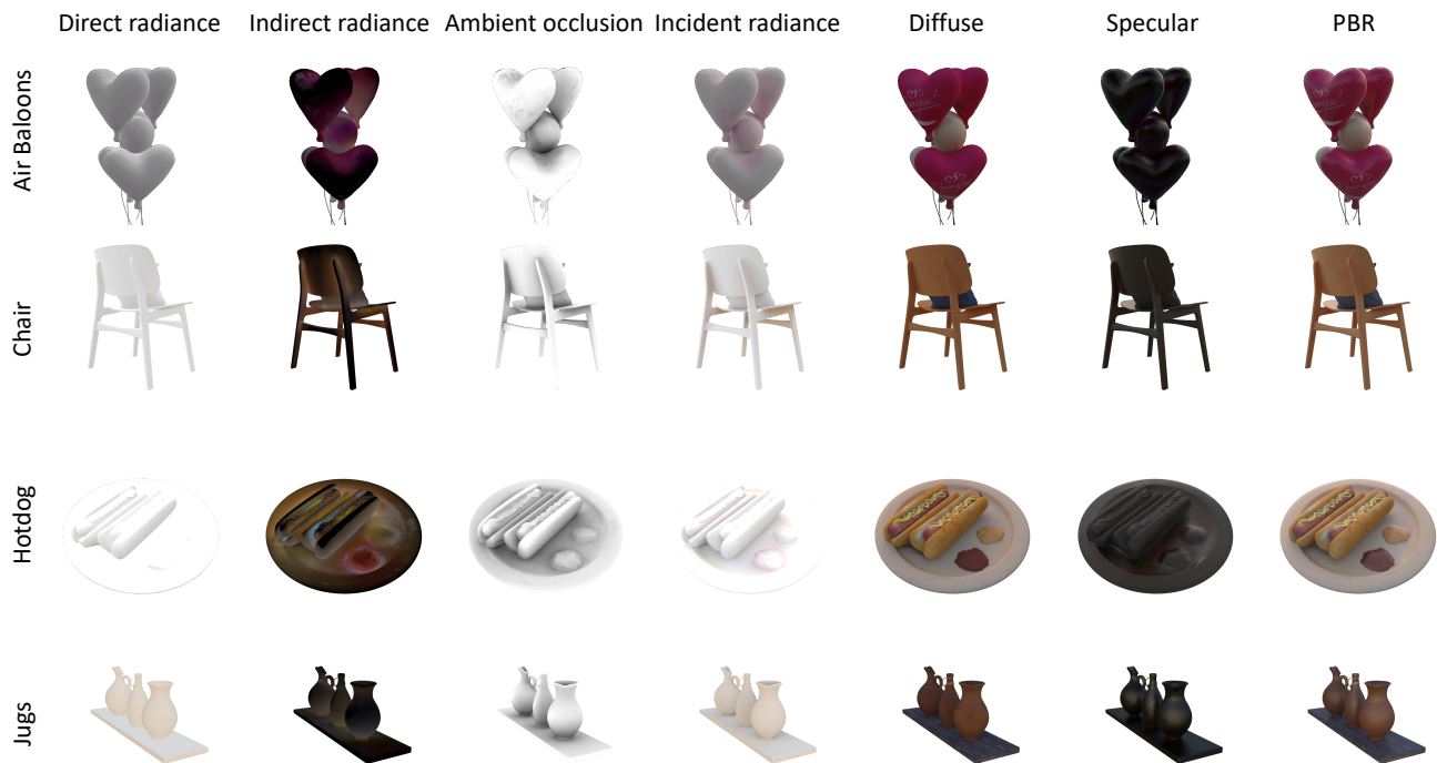
Figure 13. Visualization of estimated components in novel view, including the averaged direct radiance L_{\text{dir}} , averaged indirect radiance L_{\text{ind}} , averaged visibility V (ambient occlusion), averaged incident radiance L_i , diffuse, specular, and final PBR color.
