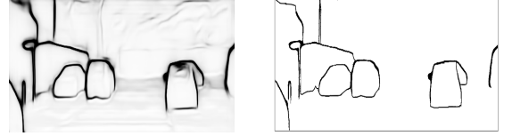
Figure D.2. Output of the edge neural network (left) and contour estimation after post-processing (right)
