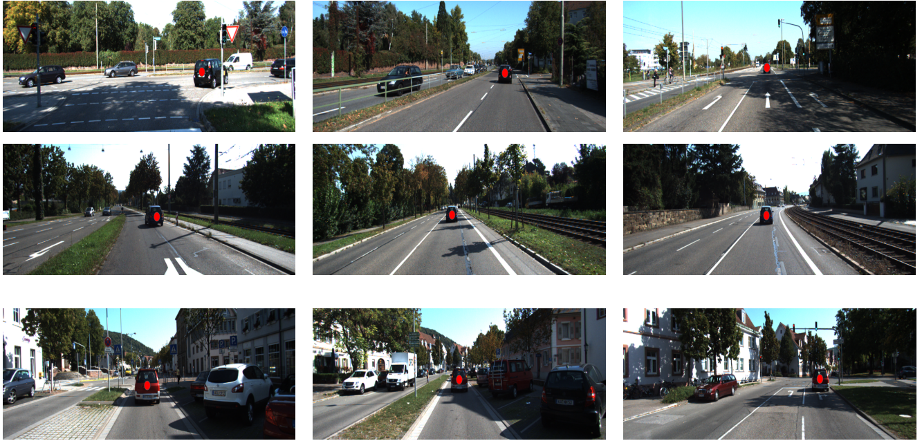
Figure F.4. Images of KITTI MOTS[72]. Each row shows a red point on the object tracked along the sequence. First row is sequence 4, second row is sequence 10 and last row is sequence 11. Timeline is arranged from left to right. Red circle is the point tracked and considered for our experiments
