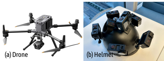
Figure 1. (a) M350RTK DJI drone for aerial images. (b) Helmet with six DJI Osmo Action4 cameras for street images
