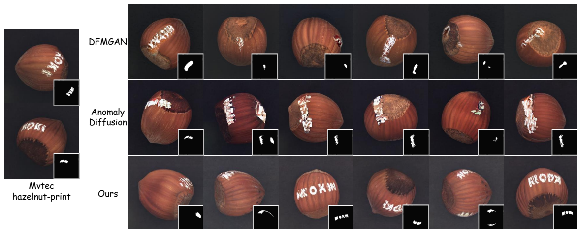
Figure 2. Comparison on the type of hazelnut-print. DFMGAN and AnomalyDiffusion struggle to generate realistic anomalies, particularly in the print class, where the anomalous regions consist of strings of letters. In contrast, our method successfully generates both the shape of the letters and the corresponding mask that aligns with their contours.
