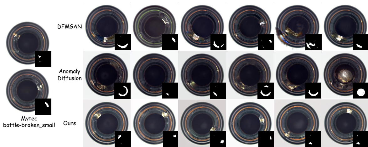
Figure 7. Comparison on the type of bottle-broken_small. This type of anomaly refers to a small blemish around the edge of a bottle, while broken_large indicates a larger blemish in the same area. The quality of the image generated by DfMGAN is limited, and the mask are not properly aligned. while the abnormal position generated by AnomalyDiffusion sometimes is not correct, and the shape does not belong to the type of broken_small, but more like broken_large. Our method, however, achieves good results in both position and shape.
