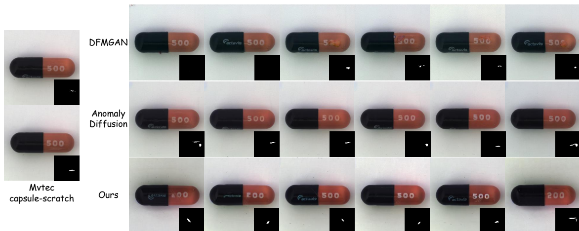
Figure 6. Comparison on the type of capsule-scratch. For scratches, a relatively minor type of anomaly, neither DFMGAN nor AnomalyDiffusion can generate effective results. In contrast, our method not only produces realistic anomalies but also demonstrates a good variety.
