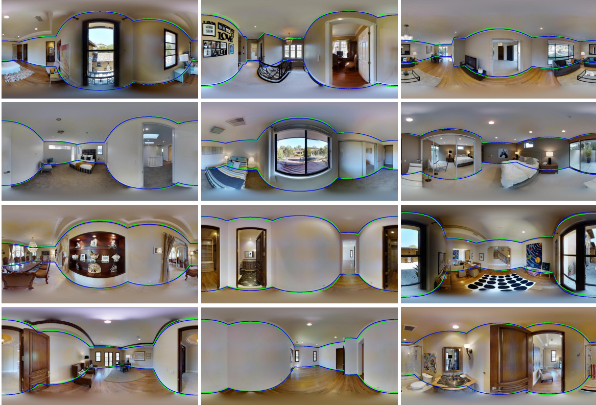
Figure 5. HUSH framework-based layout estimation. Blue and green lines represent ground truth labels and our predictions respectively.
