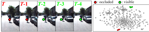
Figure S-4. t-SNE visualization of features for regions occluded by moving objects.
