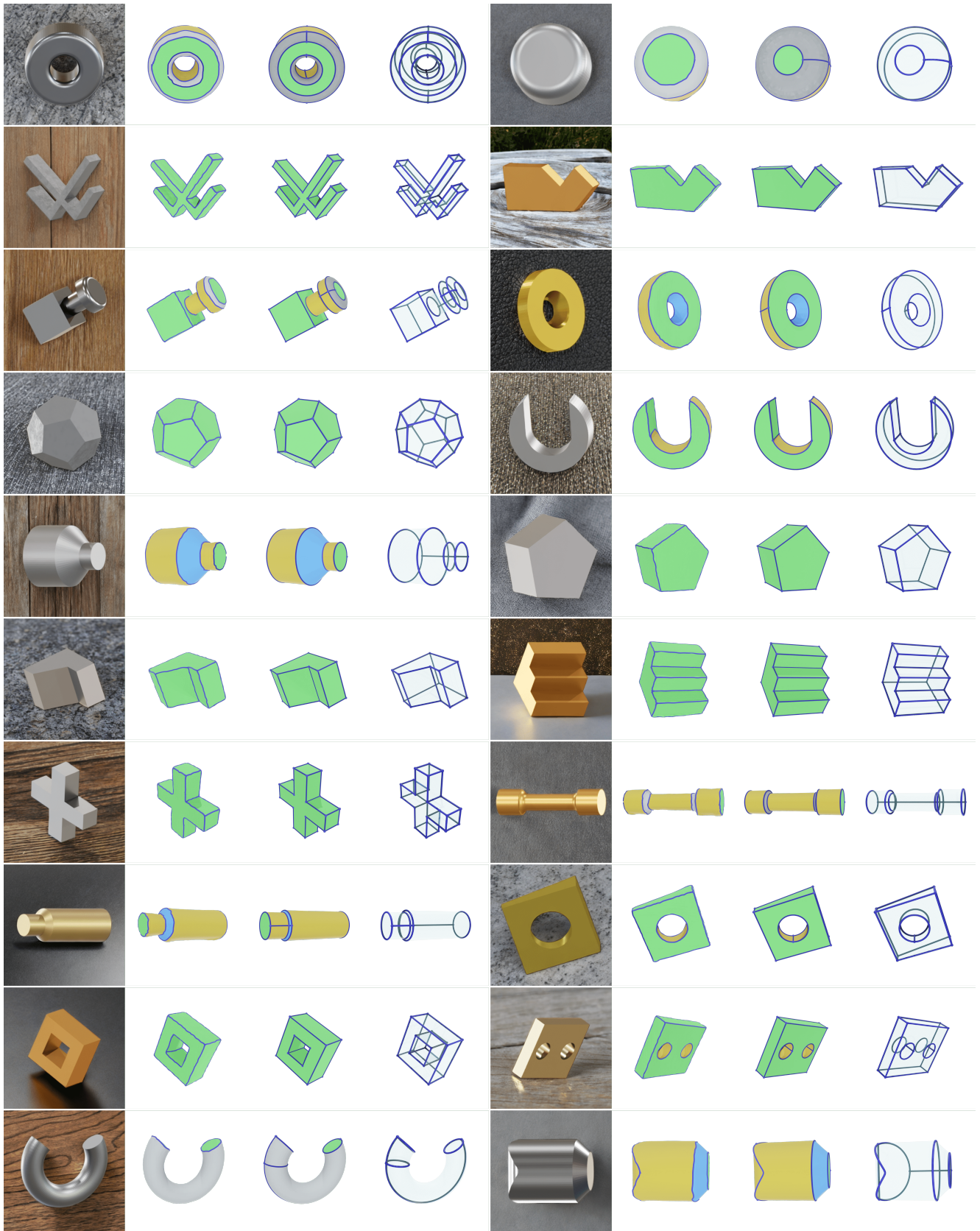
Figure A5. Reconstruction results from the given images are shown from left to right: input image, reconstructed mesh, B-reps, and their CAD vertices and edges. Different colors indicate different primitives: plane (green), cylinder (yellow), cone (blue), sphere (pink), and torus (grey).
