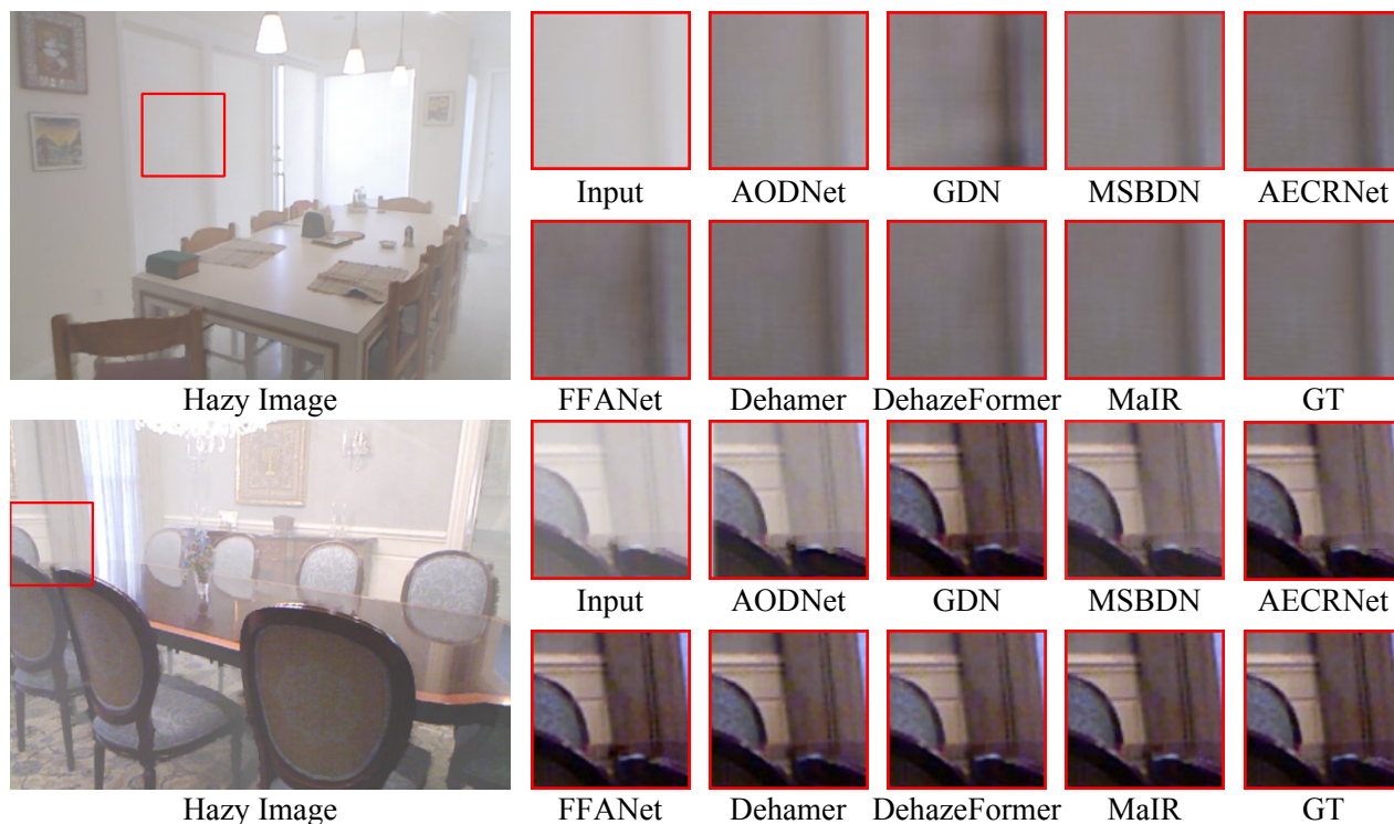
Figure 4. Visual comparison of image dehazing results on the SOTS dataset. MaIR can effectively remove haze and restore contents with colors that closely match the ground truth.
