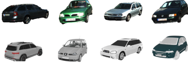
Figure 8. Pose matching results. It shows that the pose of retrieved CAD models (second row) can match accurately with the pose of the input vehicle images (first row) despite the large difference between appearance and geometry.
