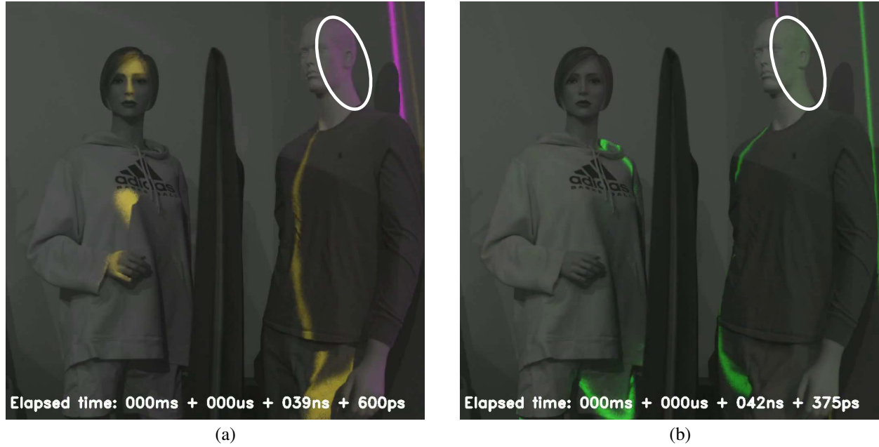
Figure C.3: 2-bounce indirect reflections in Figure 1 scene. (a) Indirect light transport on the mannequin face from the magenta laser. (b) Indirect light transport on the mannequin face from the green laser.
