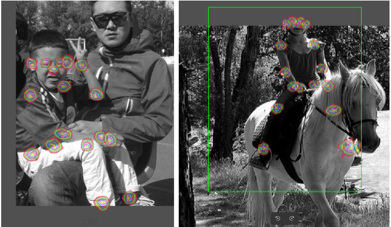
Figure 13. Calibrated probability maps with probability levels thresholded in 10% steps. Each color represents area with 10% probability that the keypoint is in that area. The green area in the right image shows activation window (AW) area. Notice that the probability map is more precise for smaller (face in the left image) and visible (left side of the right image) keypoints.
