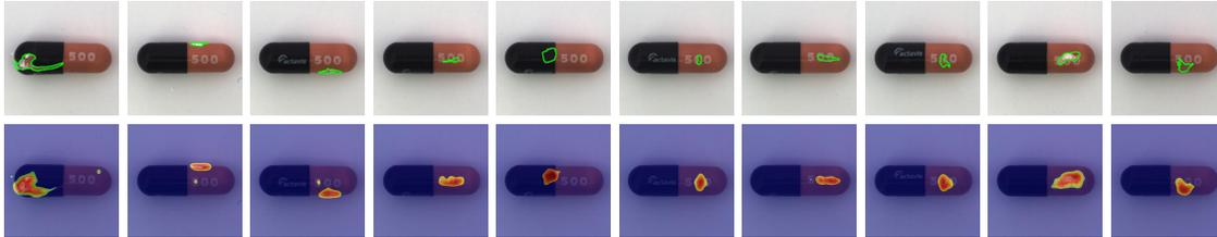
Figure A.6. Visualization of segmentation results for the capsule category in MVTec-AD. The first row represents the input images, with green outlines indicating the ground truth regions. The second row shows the results of anomaly segmentation.
