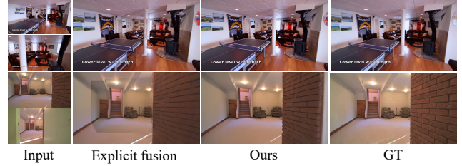
Figure 5. Qualitative results on ablating different fusion strategies. GEN3C can generate a realistic novel view with misaligned depth and different lighting in the input views, while the explicit fusion strategy fails.
