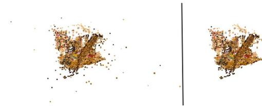
Figure 7. A comparison of the SfM point cloud before and after filtering on the “playroom” scene of the Deep Blending dataset. The point cloud on the left represents the pre-filtered state with 37,005 points, and the point cloud on the right represents the post-filtered result with 36,850 points. In comparison, the right side has fewer noisy points than the left side.
