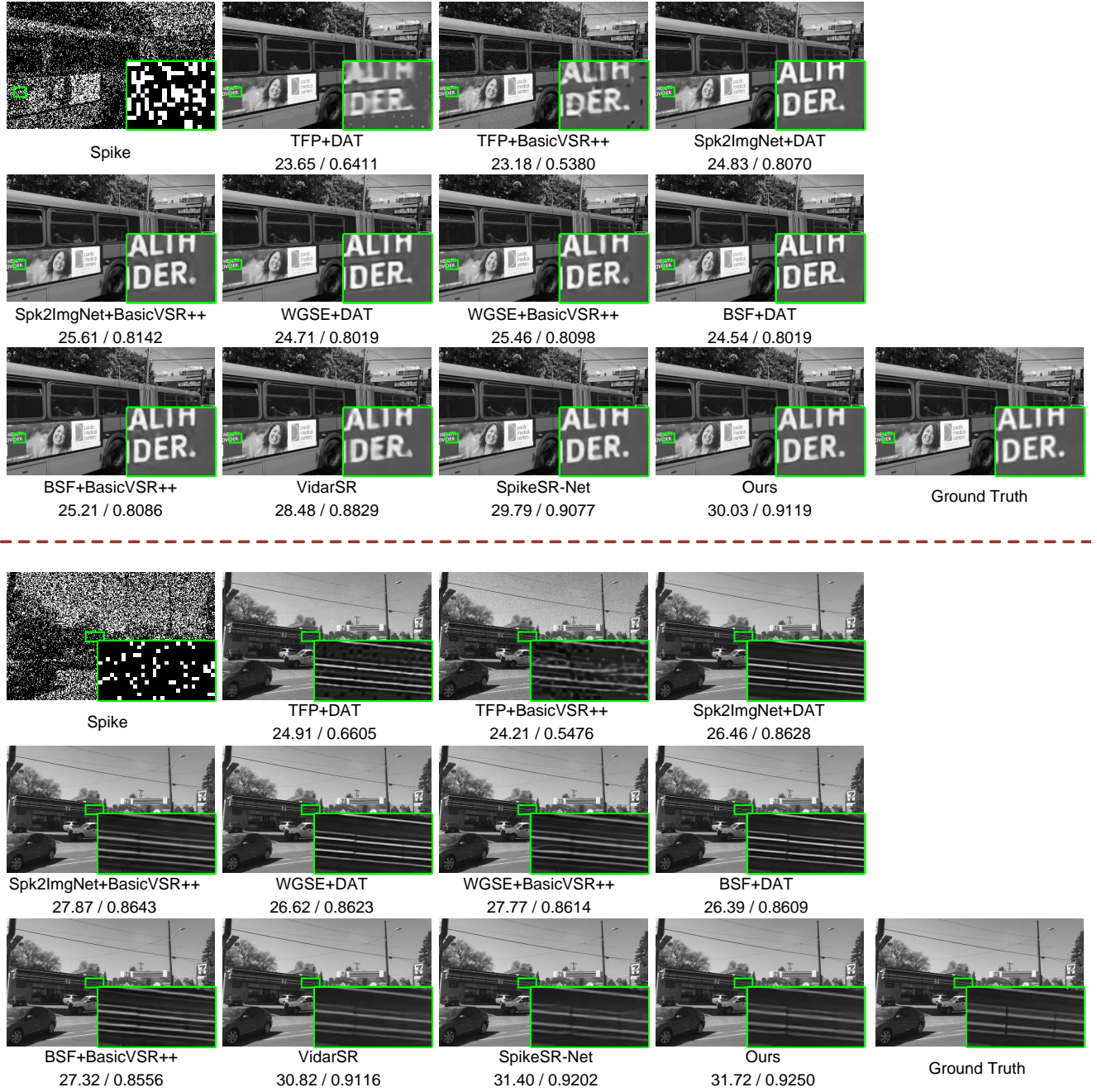
Figure 17. Visual comparison ( \times 4 ) on the Adobe240-based spike data. The values below each image represent “PSNR / SSIM” metrics. Please enlarge the figure for better comparison.
