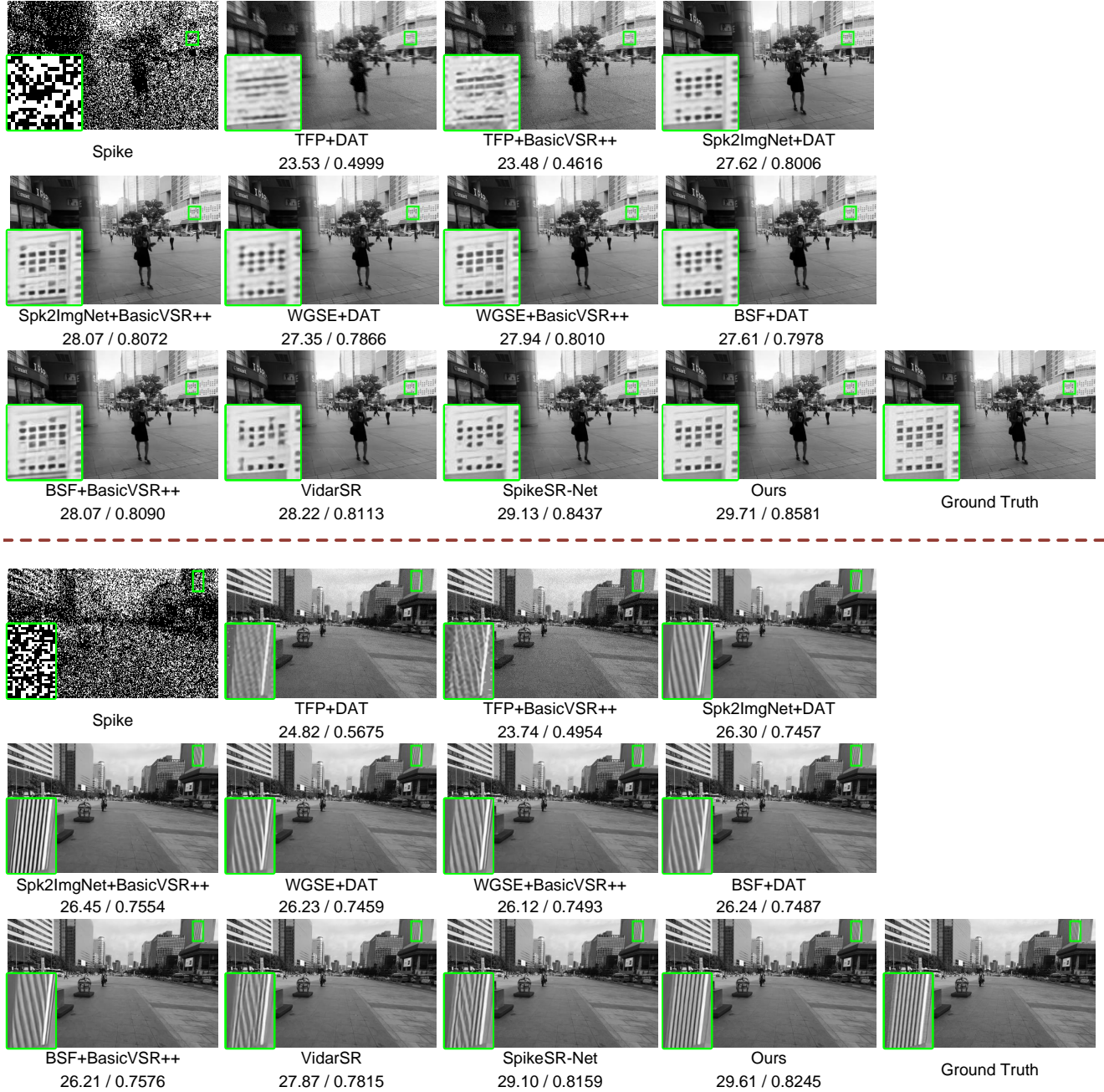
Figure 15. Visual comparison ( \times 4 ) on the REDS-based spike data. The values below each image represent “PSNR / SSIM” metrics. Please enlarge the figure for better comparison.
