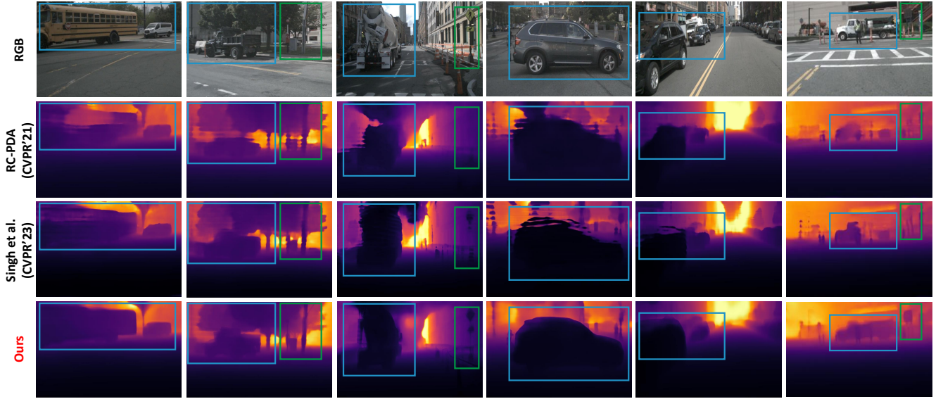
Figure 6. Visual results on daytime scenes. Previous multi-stage methods [9, 13] exhibit disrupted structures, blurred details, or noticeable artifacts. Our TacoDepth can predict accurate depth with complete structures and fine details. Best view zoomed in on-screen.
