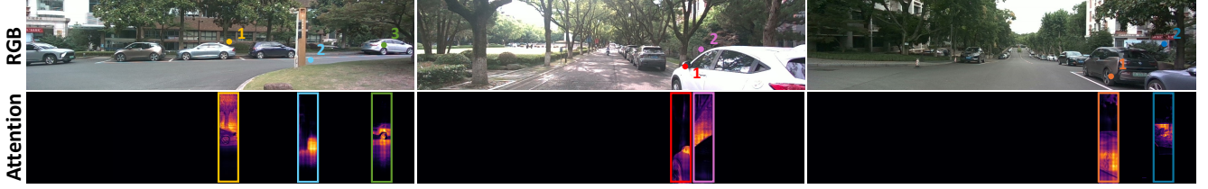
Figure 2. Visualization of attention maps. Some accurate Radar points are projected onto the image plane, as indicated by the colored points and indices. For each Radar point, the attention computation is confined to Radar-centered areas to maintain efficiency. In the attention maps, brighter colors represent higher attention scores. Our Radar-centered flash attention can effectively focus on correct corresponding regions and establish cross-modal correspondences. The attention maps also accurately distinguish between foreground and background, e.g. , shrub , road surface , car body , side mirror , stone tablet , car rear , and billboard . Best view zoomed in on-screen for details.
