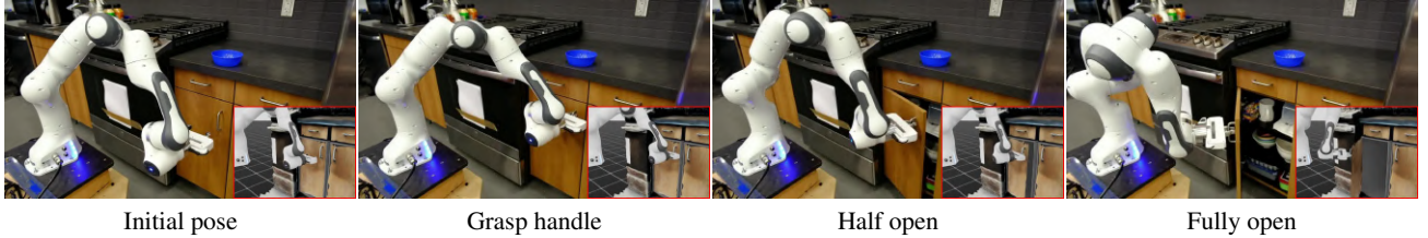
Figure 2. More Results on Real-to-Sim-to-Real. Here we showcase the robot opens the cabinet door with the revolute joint in a zero-shot transfer setting. DRAWER allows us to learn training robotic controllers using a real-to-sim-to-real loop. The inset images indicate the simulated data generation process.
