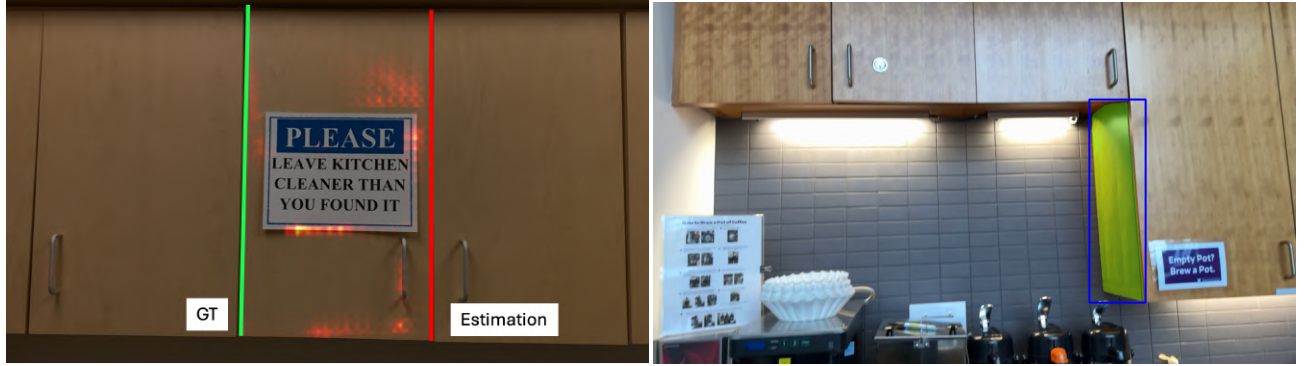
Figure 9. Failure cases of DRAWER. DRAWER might occasionally fail due to catastrophic errors in foundation models. For example, when 3DO1 predicts the wrong axes and GPT-4o fails to recognize the correct face of cabinet doors.
