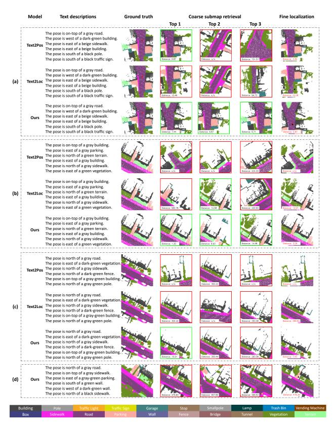
Figure 10. Qualitative localization results on the KITTI360Pose dataset: In coarse submap retrieval, green boxes indicate positive submaps containing the target location, while red boxes represent negative submaps. For fine localization, red and black dots correspond to the ground truth and predicted target locations. We label the distances between the prediction and ground truth in the submap, with "n/a" indicating submaps from different scenes.
