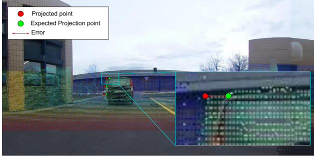
Figure 12. Illustration of LiDAR point projection onto an equirectangular image. The red dots represent the projected points from LiDAR data, while the green dots indicate the expected projection points on the image. The red arrows show the pixel-wise error between the projected points and the expected points, which is used to quantify the projection accuracy. This error metric aids in evaluating the fidelity of LiDAR-to-image projection in the HELVIPAD dataset.
