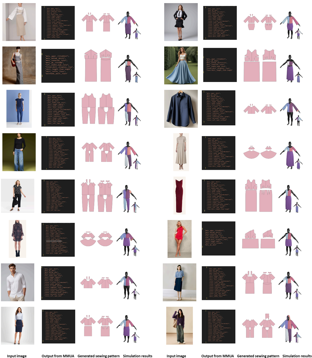
Figure 16. Additional Image-guided generation results. From left to right: input image; output from MMUA; generated sewing pattern; simulation results.
