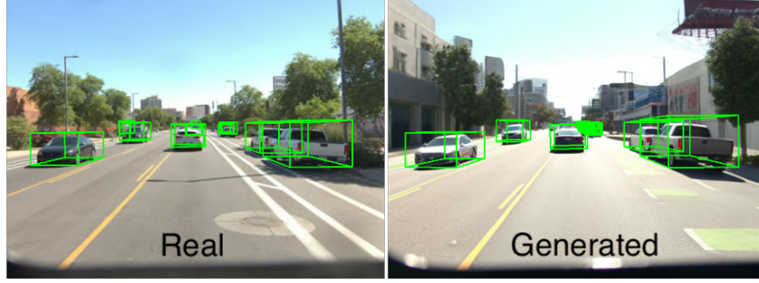
Figure 3. Comparing detection results on real logs and synthetic images generated by SceneCrafter.
