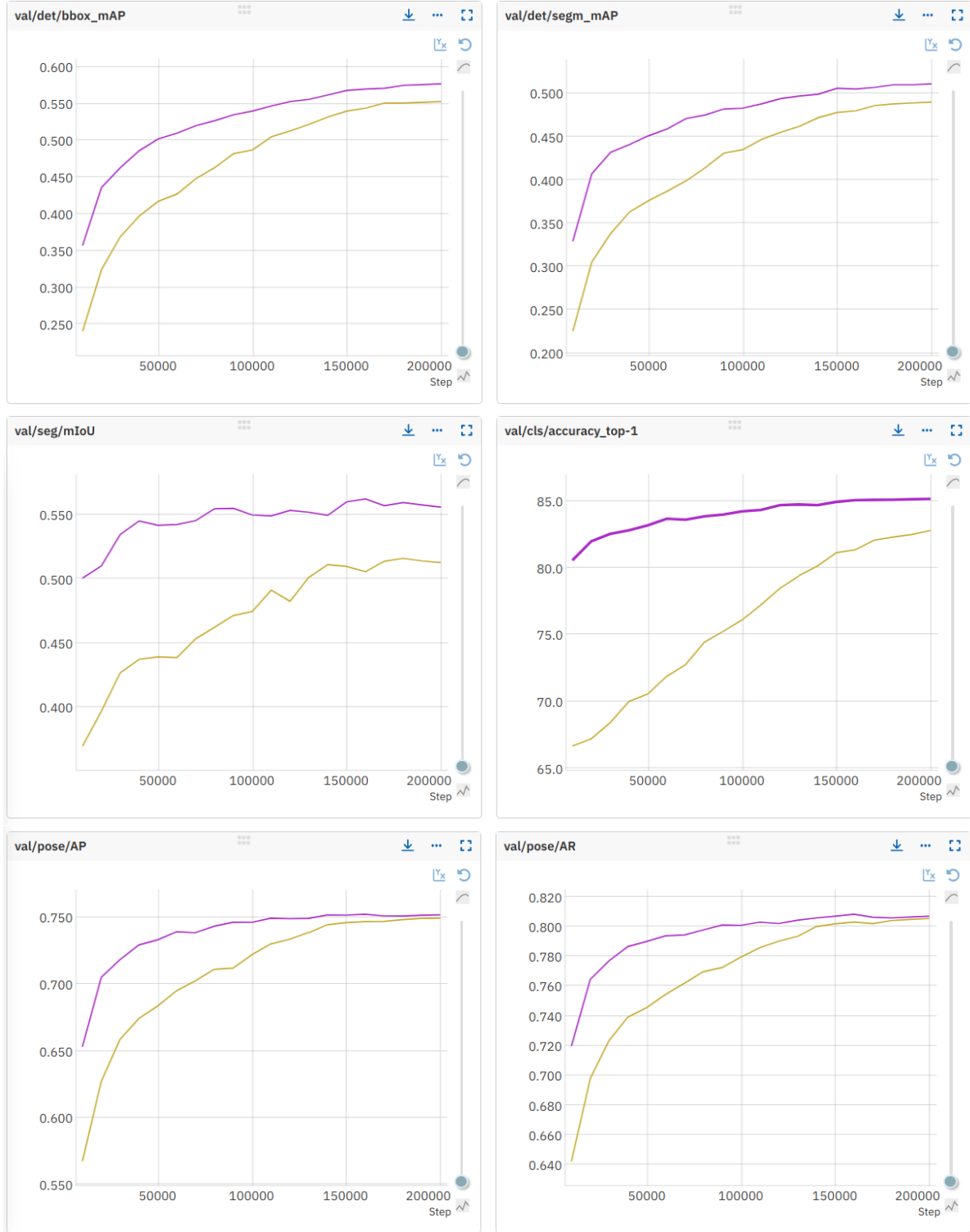
Figure 5. The validation performance of freezing ViT (the purple curve) vs. without freezing ViT ( i.e. training all parameters, the yellow curve) in multitask pretraining of 5 tasks. Freezing ViT converges much faster and achieves higher performance in the end of training. The tasks are annotated with labels: object detection (det/bbox_mAP), instance segmentation (det/segm_mAP), semantic segmentation (sem/mIoU), classification (cls/accuracy_top-1), pose estimation (pose/AP, pose/AR).
