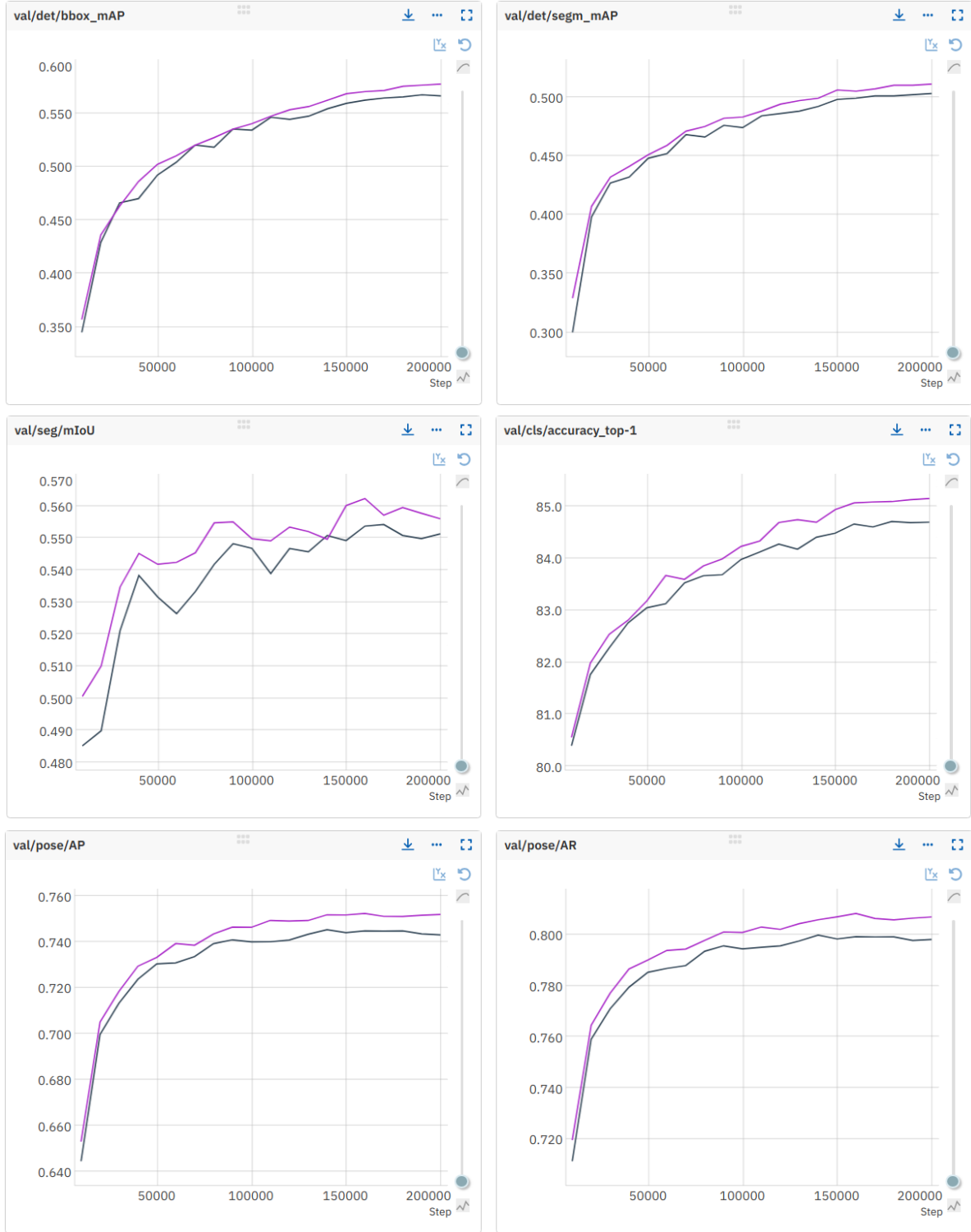
Figure 6. The validation performance of BN (the gray curve) vs. GN (the purple curve) in the 5-task MTL training. GN consistently outperforms BN in all tasks. The tasks are annotated with labels: object detection (det/bbox_mAP), instance segmentation (det/segm_mAP), semantic segmentation (sem/mIoU), classification (cls/accuracy_top-1), pose estimation (pose/AP, pose/AR).
