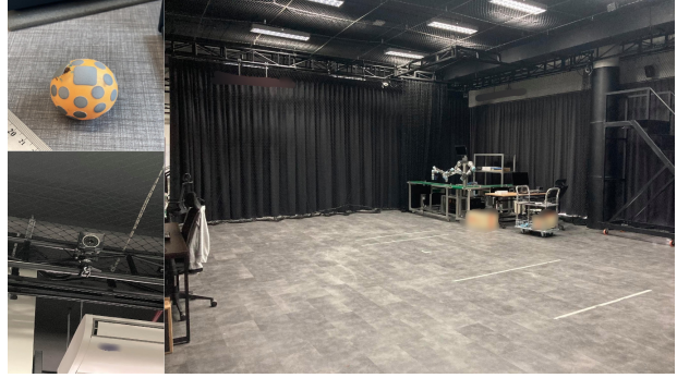
Figure 10. Motion capture studio. The top left is a ping-pong ball attached with IR reflective materials. The right image is our motion capture studio used to collect data. The bottom left is one of the eight IR cameras used in the studio.
