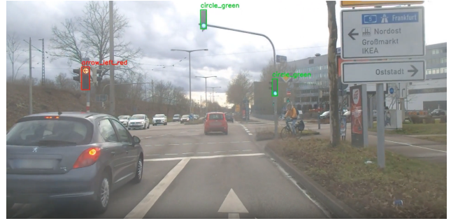
Figure 5. Example for traffic light detection and state recognition using the fine-tuned YOLO model provided by KASTEL-MobilityLab’s. The model is capable of detecting direction specific traffic lights.
