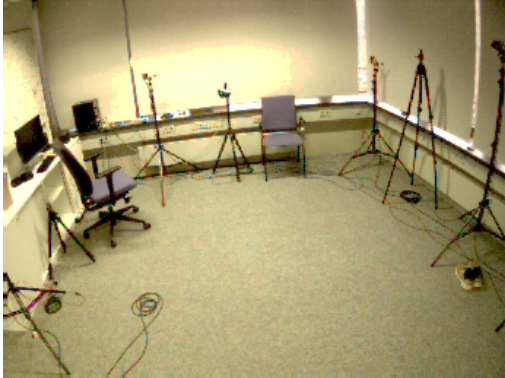
Figure 7. Our portable setup in one of the recording rooms. It consists of six hardware-synchronised iniVation DAVIS 346C colour event cameras on tripods, connected to a workstation with 10 m optic fibre USB3 extension cables. We installed two additional PCIe USB3 extension cards into the workstation to connect all cameras with the required bandwidth.
